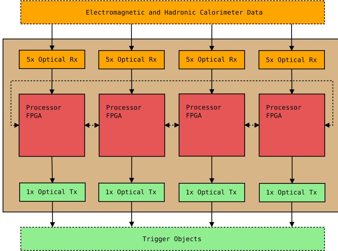
Figure 2.5: Real-Time Data Path of the jFEX
