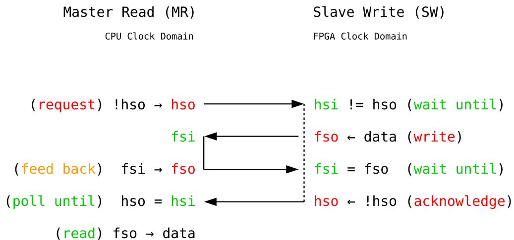
Figure 4.4: Reading From the FPGA
