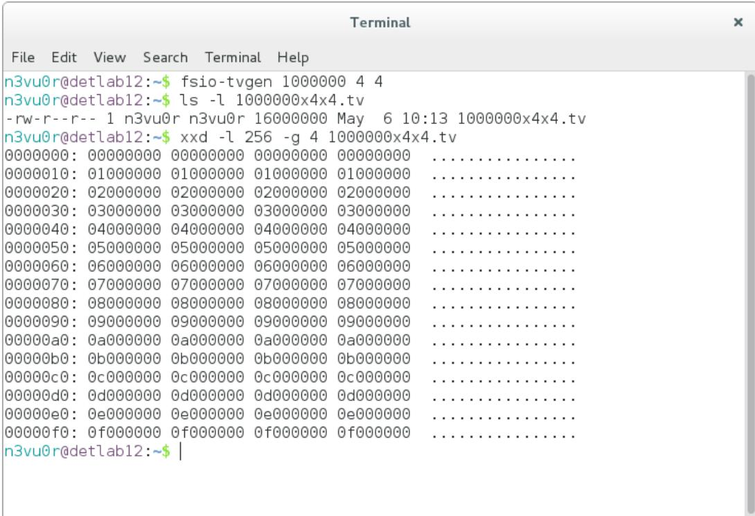
The screenshot shows a terminal window titled "Terminal". The command `fsio-tvgen 1000000 4 4` is run to generate a test vector file. The resulting file is listed with `ls -l 1000000x4x4.tv`. The file is a binary dump of memory starting at address 0x00000000, with a size of 1000000 bytes. The dump shows a repeating pattern of values from 0x00000000 to 0xffffffff. The terminal window has a standard Linux-style interface with a menu bar and a scroll bar.
