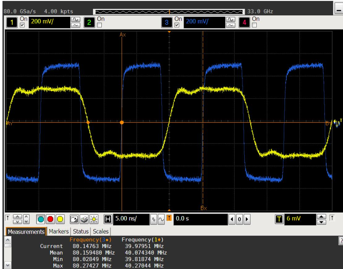
Figure 5.20: Doubled Clock Frequency [73]
