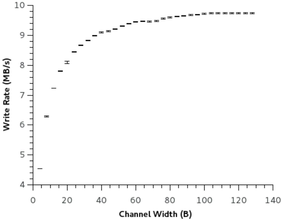
Figure 5.7: Write Rate vs. Channel Width
