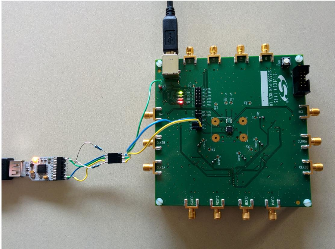
Figure 5.12: Control via External I<sup>2</sup>C Module [63, 54]
